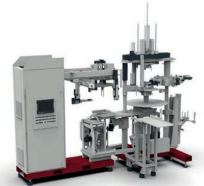
Winding and inserting centers
